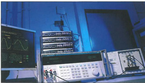
A commercial high-precision calibrator (center) is being calibrated by means of the AC quantum voltmeter in the AC voltage mode.
